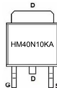
Marking and pin assignment
