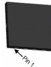
DFN 3.3x3.3 EP top view
